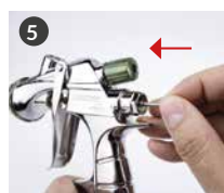
Insert the needle.
