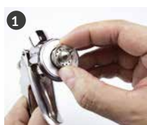
Assemble the fluid nozzle.
