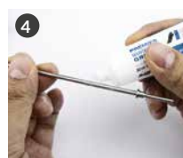
Grease the needle (code W2COM6165).
