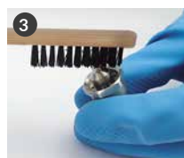
Clean the tip of the nozzle carefully with a brush (code W2COM6163).
