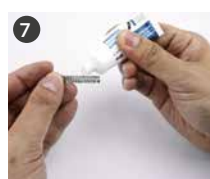
Grease the Needle spring.
