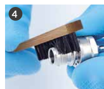
Clean also the thread of the nozzle carefully with a brush (code W2COM6163).
