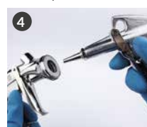
Dry with the Air blow gun.
