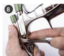
Grease the air air valve bar behind the trigger.
