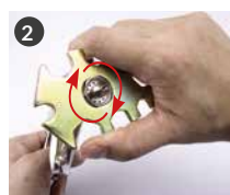
Tighten up the fluid nozzle with the universal spanner (code 930171A0).
