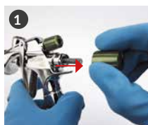
Take out the fluid adj. knob and needle spring.
