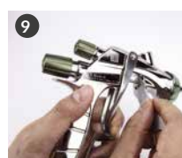
Adjust (15-60 degree tighten) the needle packing with spanner.
